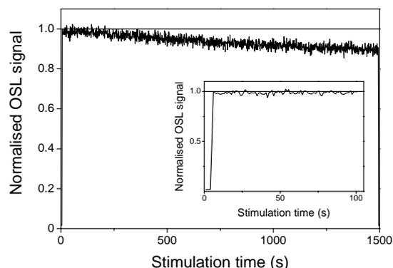
**Figure 2:** Signal observed from an annealed blank silicone-sprayed stainless steel cup during stimulation with blue diodes for 1500 s at  $250^\circ\text{C}$ ; the signal has been normalised to that observed in the first second of stimulation. The inset shows the signal observed during the first 100 s of stimulation.
