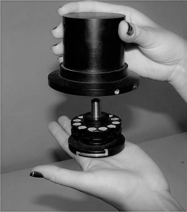
Figure 3. The sample holder, hosting up to 24 discs (below), and the container.
